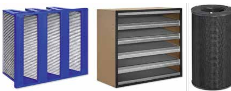
Figure 5: Carbon filter cells for the adsorption of gaseous odourous compounds, hydrocarbons and trace inorganics from recirculated air. Can fit into existing fittings and activated carbon can be tailored to application needs (i.e. use of impregnated activated carbon). Cartridge type filters (far right) are easily replaceable and easy to dispose of. Used in IAQ and HVAC applications. (Image source (Accessed 02/02/16 11:02 am): http://www.troxuk.co.uk/filter-elements-and-filter-units/activated-carbon-filters-53e6bb17af9e3274 ).
